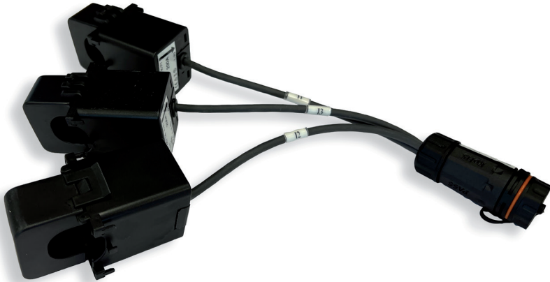
Fig. 19: Photo of sets of three current sensors 3LCT24/225 mV
